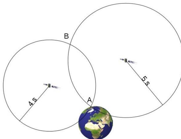
Figure 2: Configuration of two satellites. Position A on the Earth receives the signals after 4 and 5 seconds, respectively. The two signals intersect at points A and B. Since only A is on Earth, B can be discarded.
