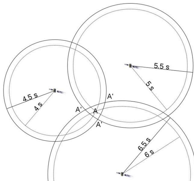
Figure 4: A third satellite is added, whose signal travel time is measured also measured wrongly. This leads to three intersections A' surrounding the true position A.
