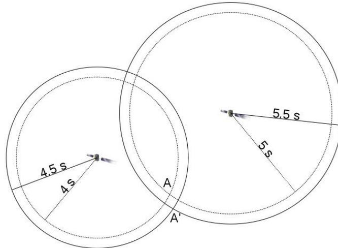
Figure 3: The same configuration as in Figure 2, but this time with a receiving clock running 0.5 s fast. Therefore, the signal transmission times are measured to be 0.5 s longer. This results in an intersection at A' instead of A.
