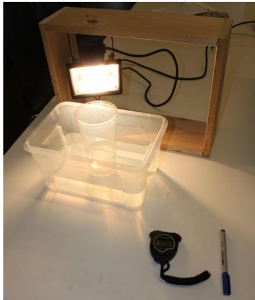
Figure 1: Experimental set-up. A plastic cup filled with water is used as a platform that carries the ice (own work).
